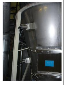
Picture right: example two mounted pneumatic impactors
